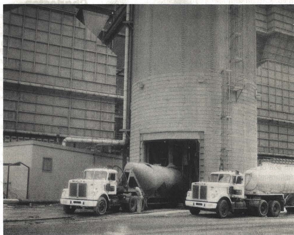
Pneumatic tanker is being loaded with dry fly ash from a silo at Clinch River Plant.
