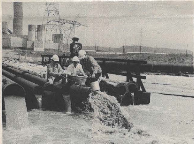
J. B. (Ben) Austin (center), professor of mechanical engineering at Bucknell and two Probers collect bottom ash samples during a test at Amos Unit 1.
