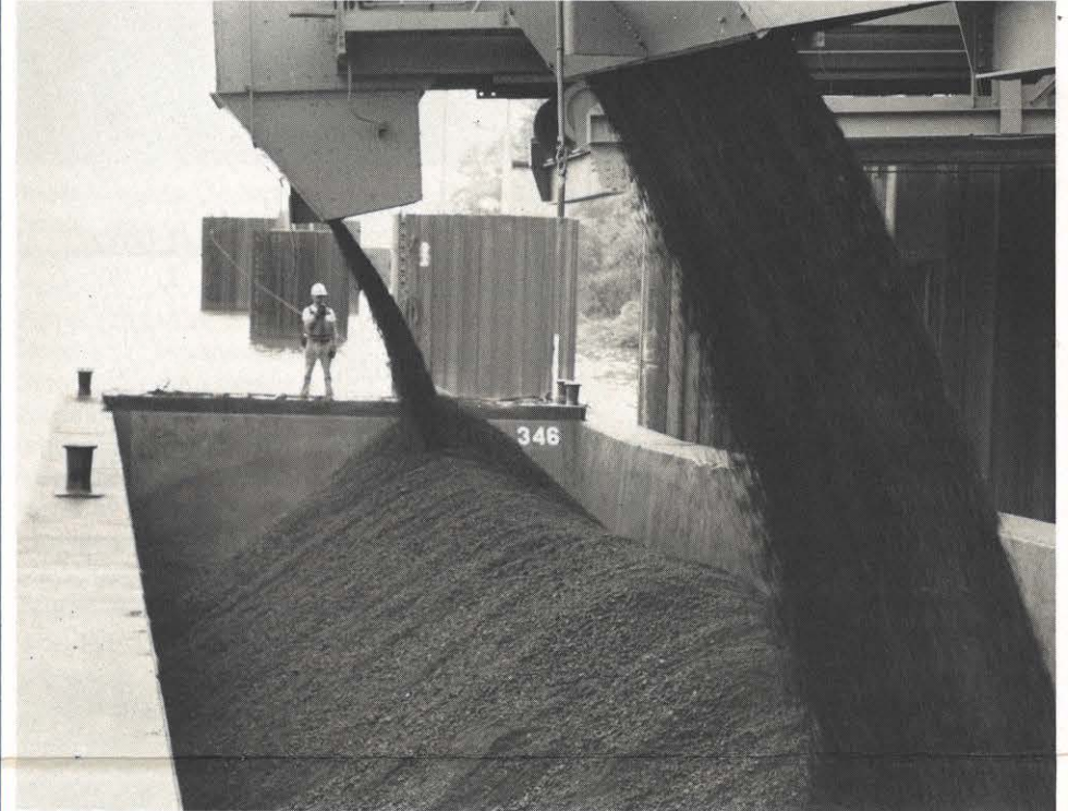
The barge loader has the capacity to load 3,000 tons of coal per hour. Thirty-four concrete cells constructed in the river allow barges to tie up securely while waiting to be loaded.
