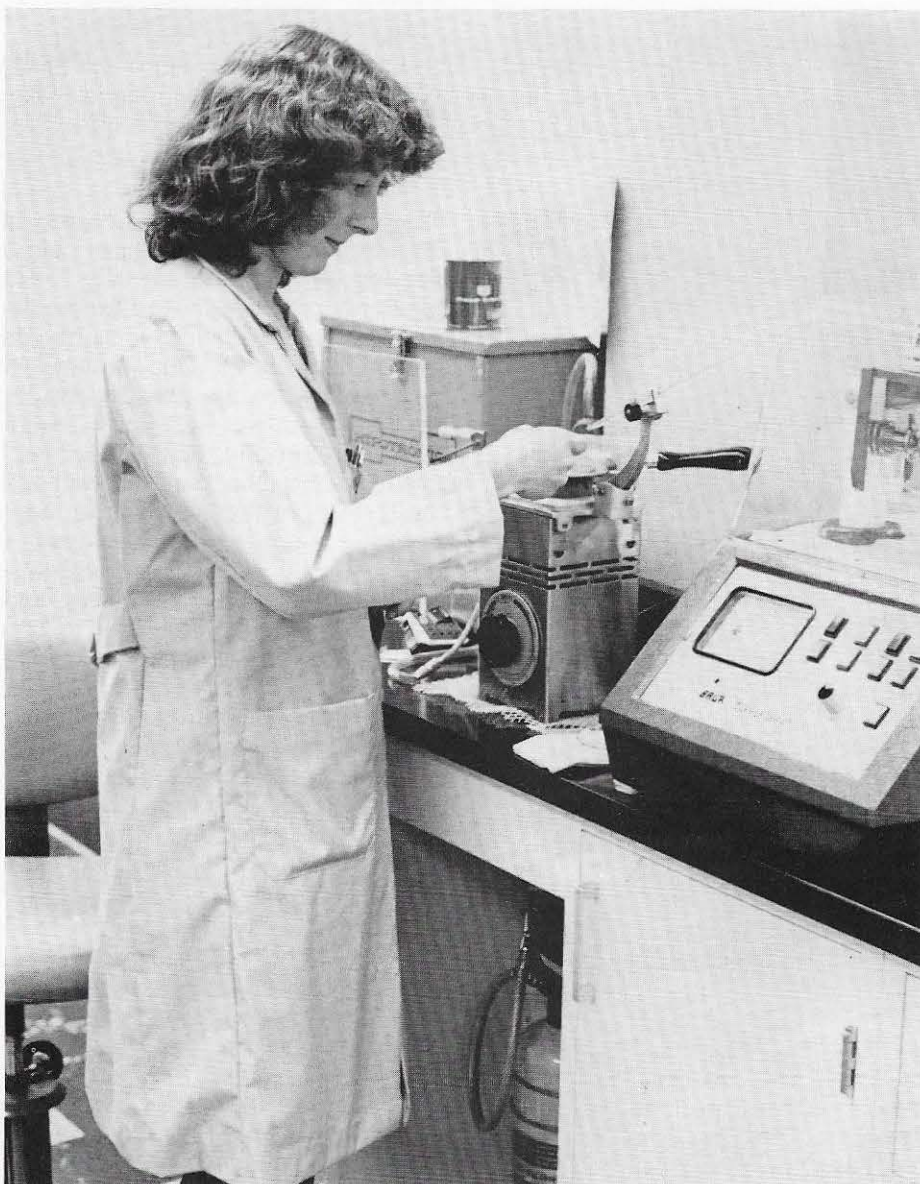
Priscilla Zeeman, engineering technician, runs test on oil to check its flash and fire points.
