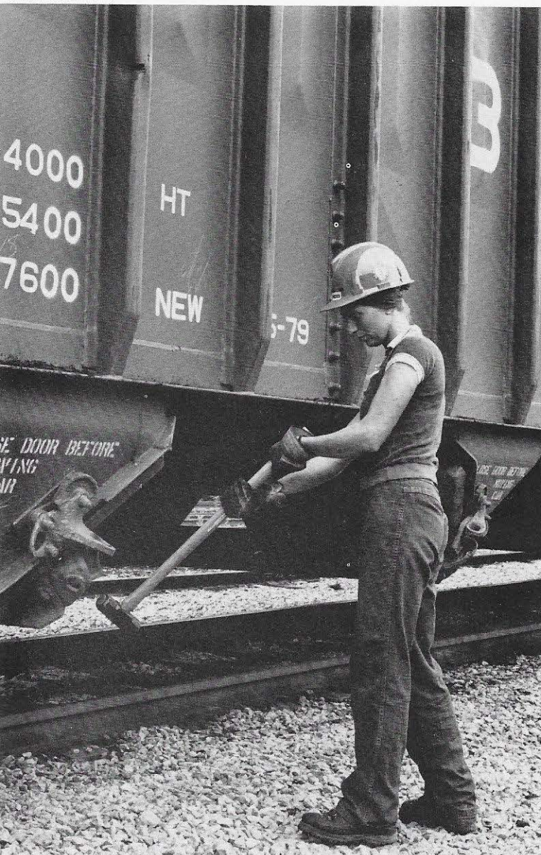
Among Angie’s duties is opening rail car doors with a 6-pound sledge hammer. She closes them with a 52 steel bar.
