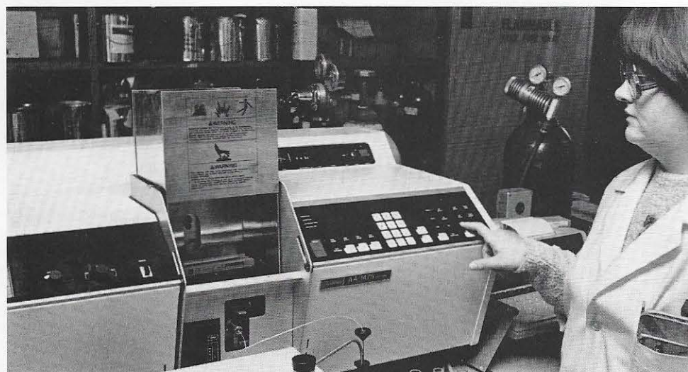
To determine trace elements in water, Jacqueline Bechtle, chemist, operates an atomic absorption spectrophotometer.
