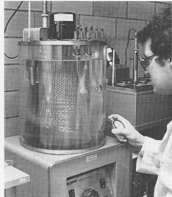
Jimmie Saunders, technician, determines the kinematic viscosity of oil. This test determines the flow characteristics of oil in system equipment.
