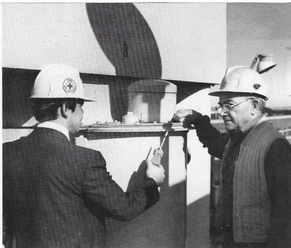
Jim Ball uses a hand-held air monitor to determine the presence of air contaminants during the checking of an equipment seal by C&SOE's George D. Davy, mechanical repairman journeyman.
