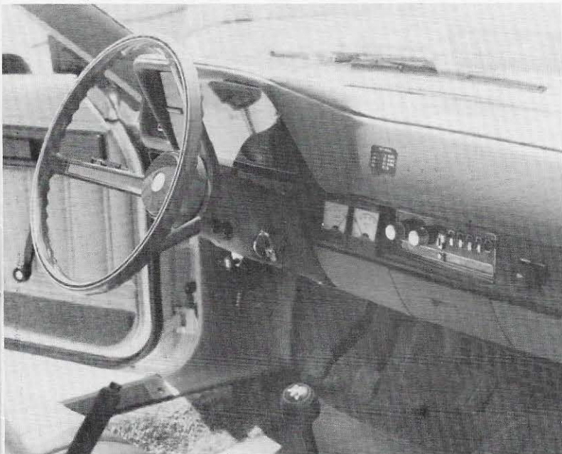
The EV dashboards have two gauges not needed by gasoline-powered vehicles. One gauge shows the amperage being drawn from the batteries and the other shows the percentage of charge still held by the batteries.
