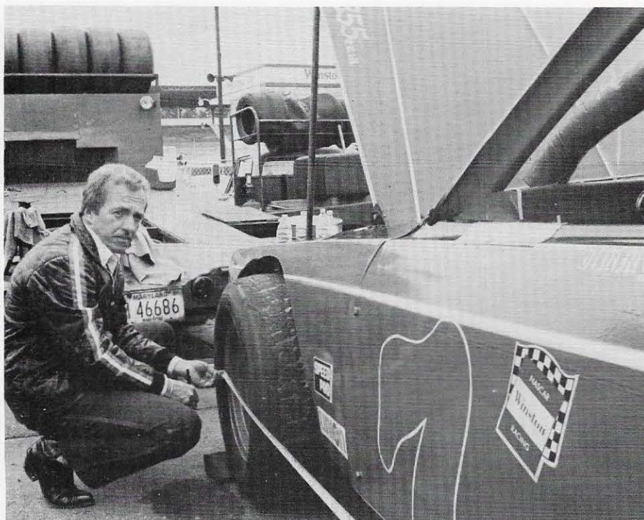
Bobby Scruggs measures the wheel base to be sure the car is not offset and meets the required length on both sides.
