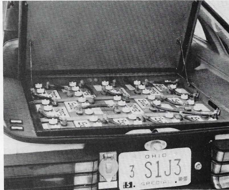
The electric car has 20 six-volt batteries located both under the hood and in the hatchback. The motor is underneath the front set of batteries. The van has a total of 17 batteries.
