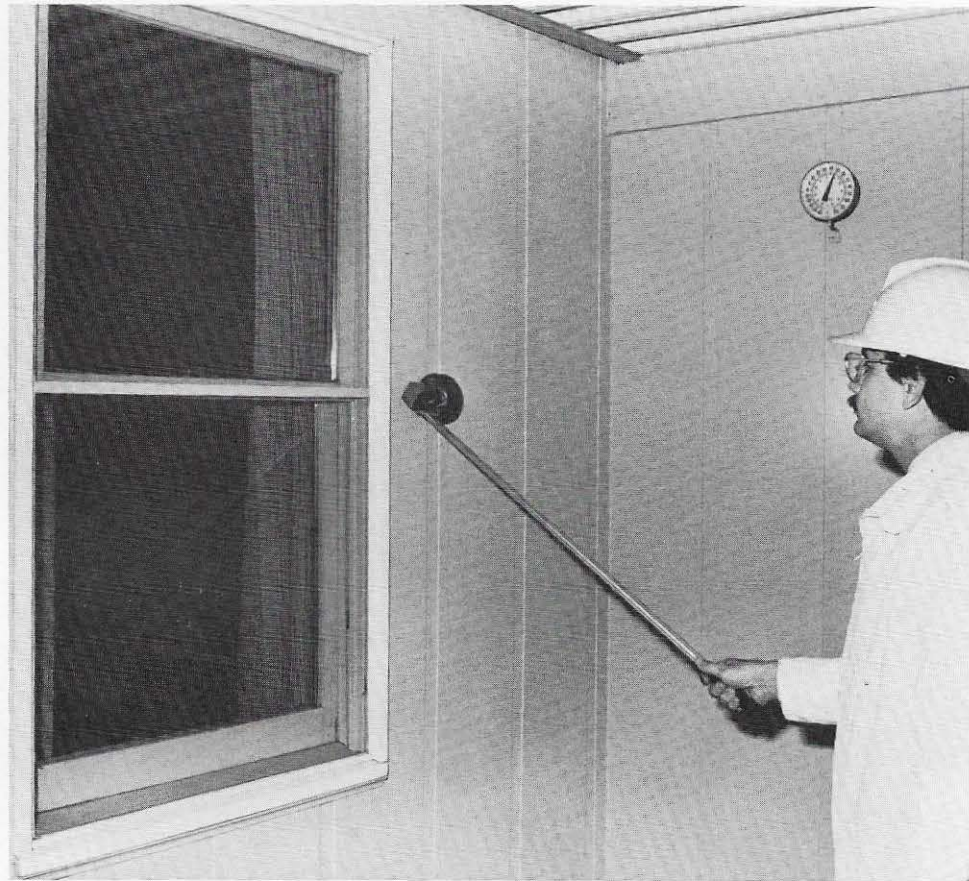
Jon Atchley, Huntington residential advisor, begins a home energy audit by measuring window areas.
