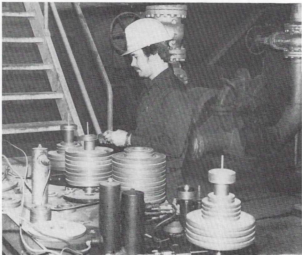
Randy Garner, performance engineer, prepares a deadweight tester to check pressure in a steam line.
