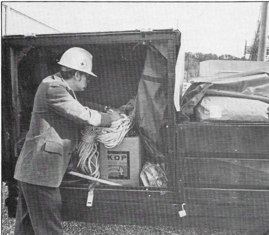
Tim Mallan, environmental engineer, inspects one of Appalachian Power's two specially equipped oil spill trailers. The trailers, located in Charleston and Roanoke, can be moved quickly to an oil spill site to be used in cleanup efforts. Tim says a quick response to oil spills is vital in order to minimize damage and cleanup costs.
