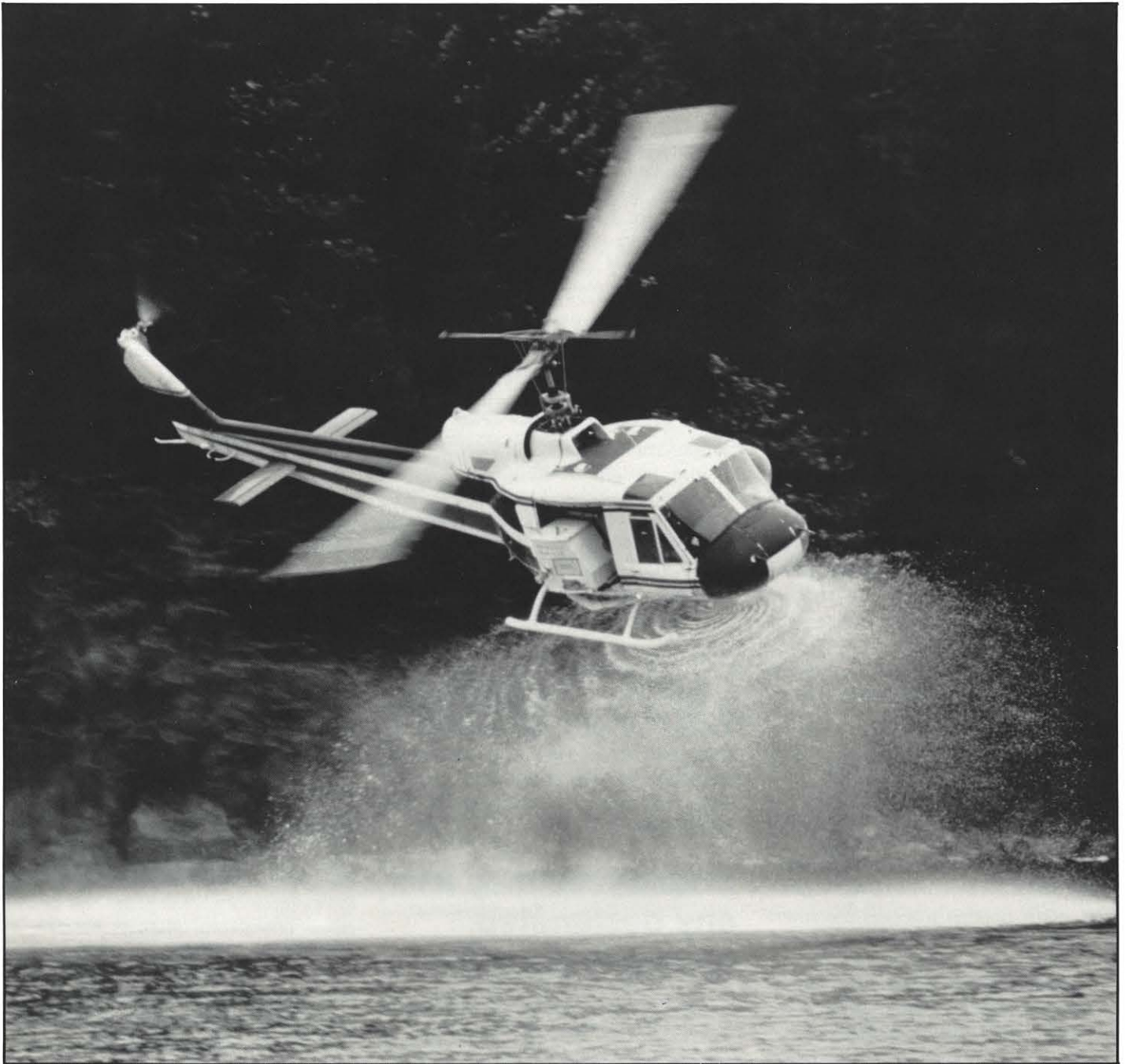
A specially equipped helicopter sprays a slurry of calcium carbonate and water on the lake's surface.
