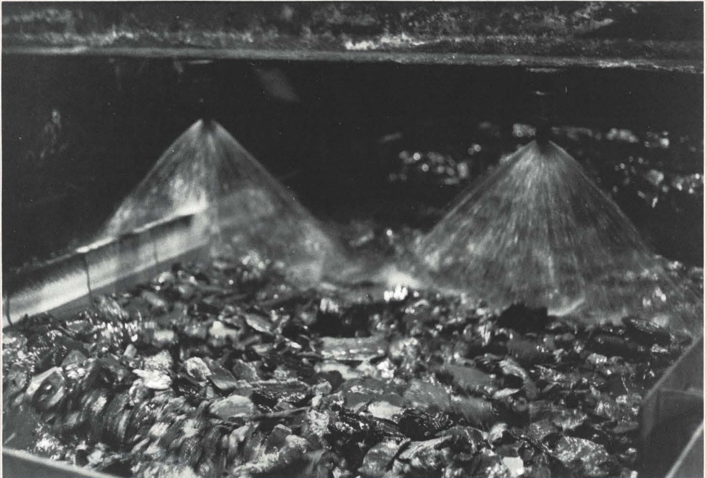
Coarse sink screens where magnetite is recovered for reuse.
