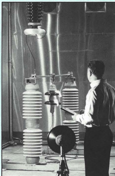
Robert Halter measures the voltage of a flashover induced on a porcelain insulator in an environmental chamber.
