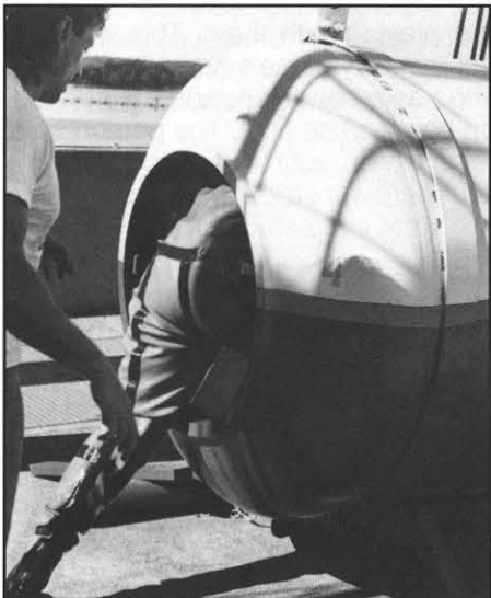
A diver enters the decompression chamber.
