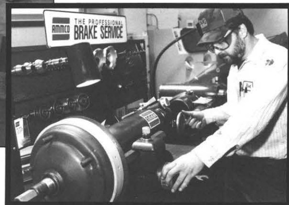
▲ Tim Crane (top photo) reams hole to install new valve guide. (Middle photo) Wayne Farley (foreground) and Bobby Paddock work on rebuilding boom on an aerial lift truck. ▶ Rodd Taylor turns a brake drum on the brake lathe.
