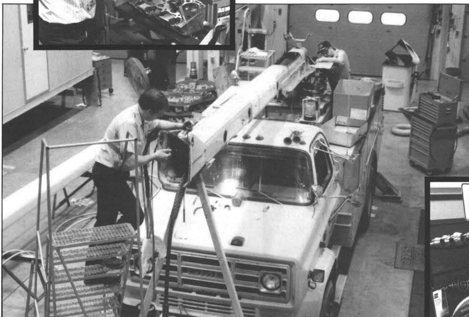
▲ Tim Crane (top photo) reams hole to install new valve guide. (Middle photo) Wayne Farley (foreground) and Bobby Paddock work on rebuilding boom on an aerial lift truck. ▶ Rodd Taylor turns a brake drum on the brake lathe.
