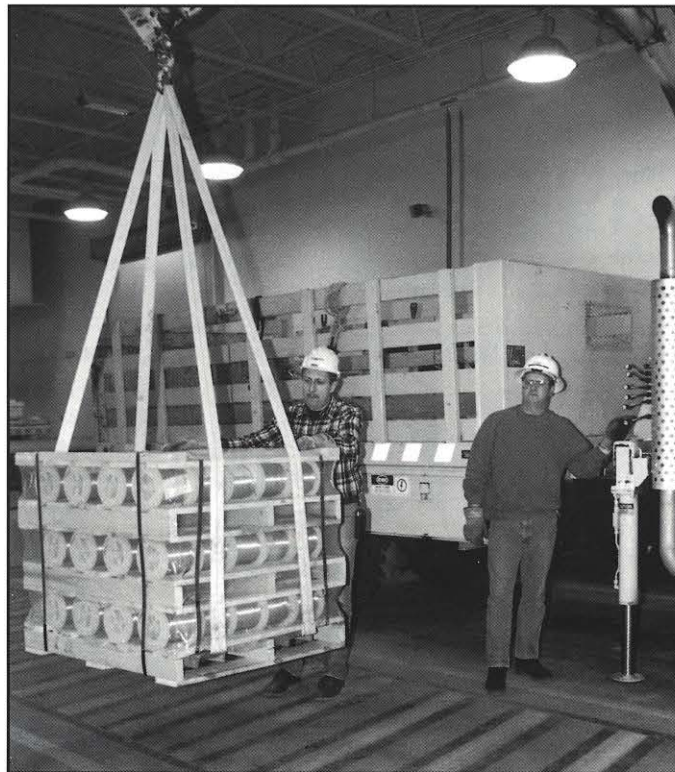
Steel channels used as lifting support to transfer a pallet or piece of heavy equipment directly from the dock to a truck were an Operating Idea from Pulaski.
